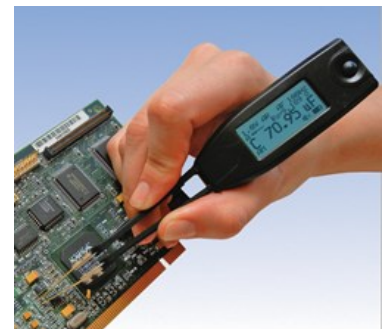
Smart Tweezers LCR-meter simplifies PCB debugging
