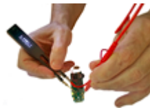
LCR-Reader 2-wire Shielded Probe Connector extends the reach of LCR-Reader's probes
